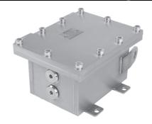
The Nautilus is a terminal enclosure that combines Ex e hazardous area certification with an unparalleled level of ingress protection. Primarily designed for submersible applications. The Nautilus is certified IP68 at 100 metres for five days to EN60529.
