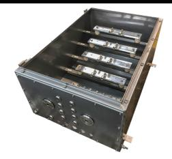
This high-current enclosure offers enhanced flexibility using a range of tinned copper busbars mounted in a tiered arrangement. The SX busbar provides termination for cables carrying up to 3000 Amps. The arrangement of busbars in this enclosure can be tailored, allowing a variety of configurations suitable for inflexible, higher-current carrying cables.
