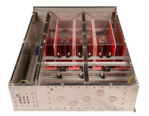
The 4TJB can accept up to three single-phase connections (one conductor per phase) in either a bottom entry or through box configuration. The -125 variants offer a unique solution for the termination of offshore umbilical cables or onshore distribution systems. In this design, the power conductor compartment houses the HV cables. A separate control compartment is used for terminating fibre optic or control cables.
