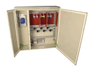
The HVJB/ABJB 125 provides a unique solution for the termination of offshore umbilical cables or onshore distribution sysems. The power conductor compartment houses connections up to 11kV. A seperate control compartment is used for terminating fibre optic or control cables.
