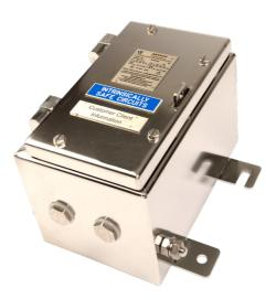
The SX range comprises of 14 standard sizes in depths of 140, 200 or 300mm. The majority can be fitted with gland plates on any or all of the four sides. Fabricated using 316L stainless steel, the SX can also be made in bespoke sizes to suit most applications.
