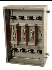
The HVJB & ABJB form the mainstay of our high voltage range, offering enhanced flexibility for choice of cables, entries and terminations. Both the 11 & 15kV versions can accept up to four phase connections, either straight through or bottom entry only. The unit accommodates up to three connections per phase.
